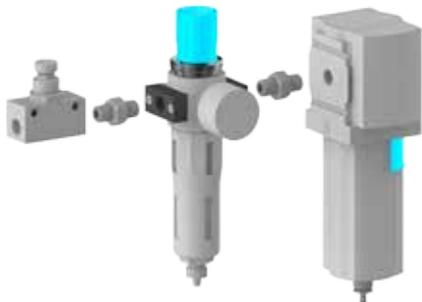
There are many benefits of using an individual filter regulator and needle valve for your AODD pump. You will always be able to run the pump with right air quality and optimum pressure and speed to save energy. Furthermore the lifetime of pump components will increase. The kit includes a filter regulator, gauge, wall bracket, needle valve, and/ or water separator. The filter is 5 micron and regulator is 0-12 bar, available in sizes 1/8" up to 3/4".
